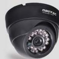
AX233 IR Dome Camera AHD & TVI Output Analog Output (Optional)
