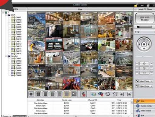
Magtec AHD DVR series is a hybrid DVR that support AHD, analog and IP camera at the same time. You can use AHD camera in places that requires high clarity. You can use lower cost analog camera in places that requires lower clarity.
